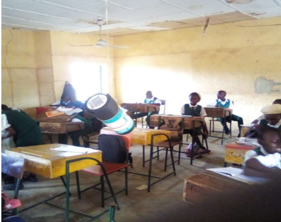
Fig. 3. Radon detector suspended at breathing height in a classroom.
