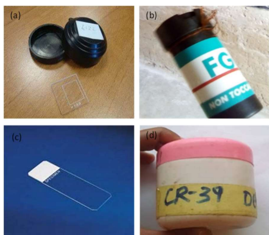
Fig. 2. CR-39 detectors and passive diffusion cups with varying dimensions used in the study.
